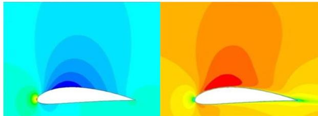
**Figure 4.** pressure and velocity plot- 0° Angle of attack
