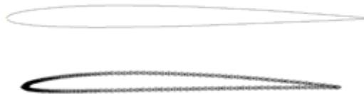
**Figure 2. NACA airfoils 1410 and 24112**
