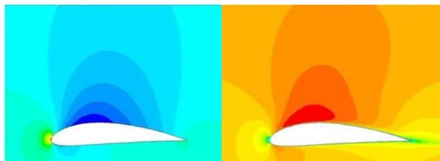
**Figure 4.** pressure and velocity plot- 0° Angle of attack
