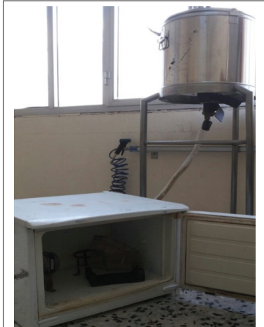
Figure 2 Set up for deep cryogenic treatment
